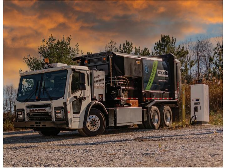
**Electric Trucks:** Since our last report, we have invested in two fully-electric refuse collection vehicles in Rutland, VT. This pilot will help us understand the potential for this technology to support our long-term fuel and emission goals. Each truck converted to electric has the potential to save on average 7,500 gallons per year of diesel fuel and prevent over 78 metric tons per year of greenhouse gas emissions.
